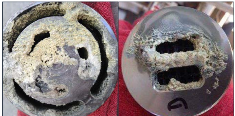
OEM valves failed due to heavy polymerization.
